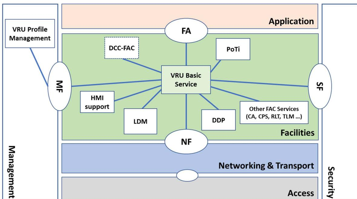
Figure 1: VRU basic service within the ITS-S architecture
