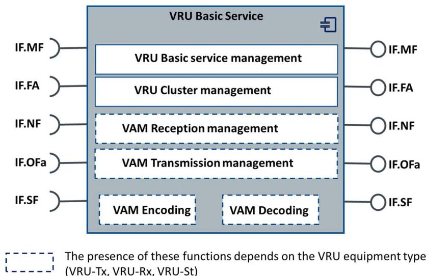
Figure 2: VRU basic service functions
