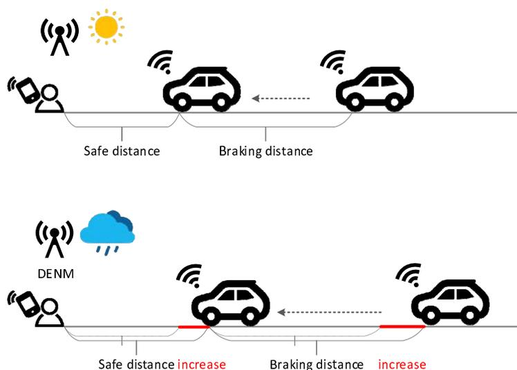
**Figure 5: Increased threshold distances after receiving DENM**
